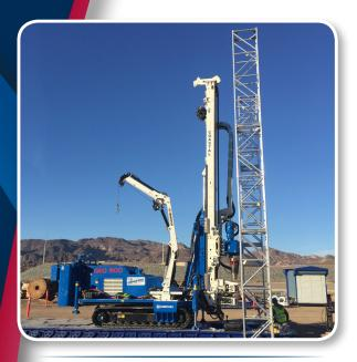
Traditional directional drilling tools rely on error based technologies that require a measurable deviation prior to making any corrections which result in a series of sweeps in and out of the desired alignment. Using Coastal's optical guidance technology, the drill operator can visually observe any deviation from the desired alignment and bring the drill bit back into alignment.
